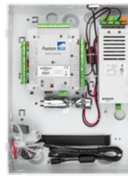
Paxton BLU Master Controller in Enclosure
